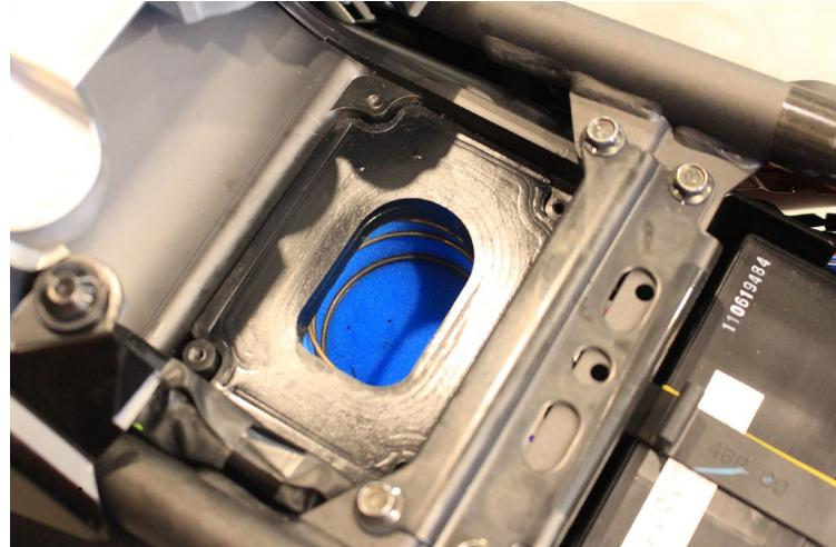
**Grease the bottom sealing edge of the air box before placing the filter into position.**
